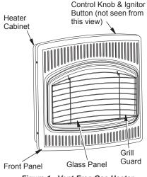
Figure 1 - Vent-Free Gas Heater
